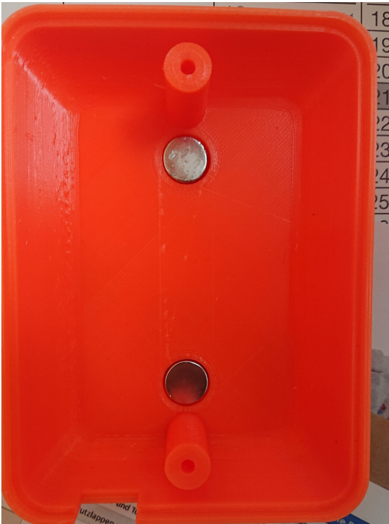
Transmitter unit: Magnets on the rear panel hold the unit in the charging station and on other metallic surfaces.
